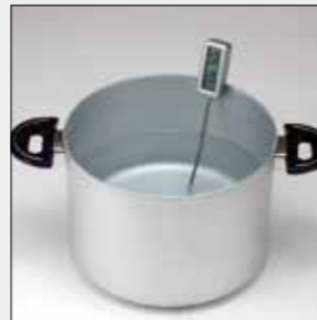
3) Dip the jaws into 55-60°C warm water.
