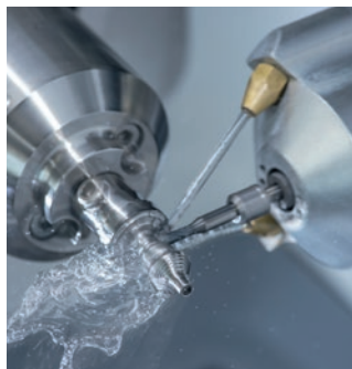
Wet processing of a Ceramill TI-Forms using the "rotational milling" technique
